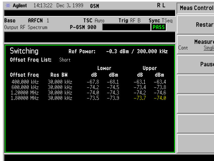
Figure 5-12 Output RF Spectrum (ORFS) Due To Switching Transients: Multiple Offset Measurement
