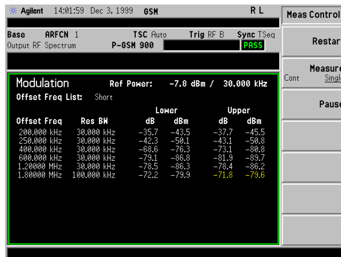
Figure 2-3 Output RF Spectrum (ORFS) Due To Modulation: Multiple Offset Measurement
